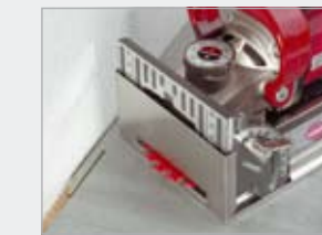
Expansion gaps (Saw blade Art. No. 132380 and slide shoe Art. No. 251057)
