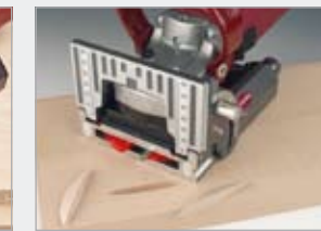
Wood repairs (Minispot cutter Art. No. 132217)
