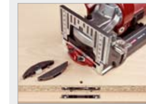
Clamex biscuit-shaped connector (8 mm cutter Art. No. 132108, drill jig Art. no. 125240 )
