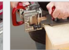
Trimming edges (Lamello Nova Art. No. 121280)
